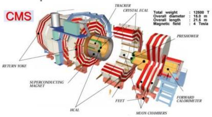
The CMS experiment is one of two large general-purpose particle physics detectors in the proton-proton Large Hadron Collider (LHC) at CERN.
